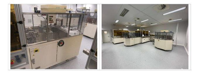
The line equipment was manufactured in 1999, installed in the factory in 2013. The line consists of 24 sections. The line has 2 flexo printers for coating, however, only one is in working order, which requires replacement of rollers and gears, and the other one needs a major overhaul. The working size of the line is GEN 1 (300x400 mm). Key equipment:
