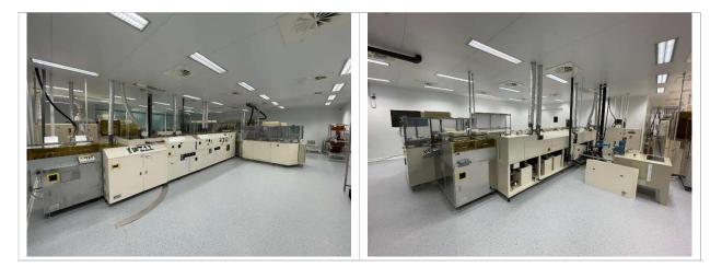
This lines equipment is mostly manufactured in 1999, installed in the factory in 2013. The line consists of 18 sections. The line includes an integrated laser structuring device MSV 2502, manufactured in 2012, designed for structuring conductive layers (ITO), without which this processing line can only be used for washing glass and plastic sheets. The working size of the line is GEN 1 (300x400 mm). The laser equipment requires replacing the old laser source with a new one. Key equipment:
