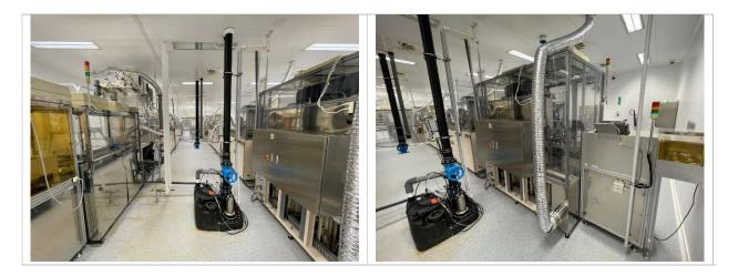
The equipment of the line was mainly manufactured in 1999, installed in the factory in 2013. The line consists of 32 sections. The line is used in the production of passive displays - smart windows, solar panels, e-ink displays. The non-vacuum aligner has been removed from the original line and placed separately and replaced in the line with more modern ODF technology, which was developed by Asymtek and the ODF equipment. The working size of the line is GEN 1 (300x400 mm). Key equipment:
