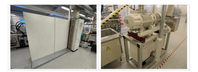
PVD coating machine for ITO, SiO2 and Nb2O5 coatings, manufacturer FHR Anlagebau (DE), 2019. PVD Machine made for reactive DC and RF sputtering, with one side load&lock chamber, maximum substrate size 1000x1500mm, for metalic, inorganic and AR coatings.
