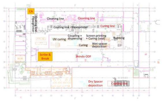
The cleanroom is managed in 4 different parts from cleanness point of view. Cleanness of class 7-8 can be reached. Highlighted in color the various cleanroom area managed separately.
