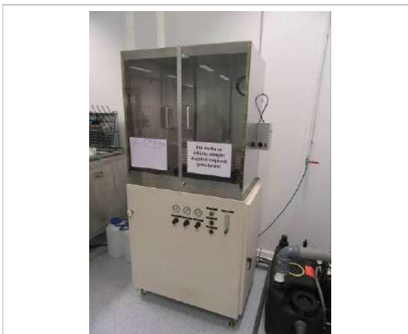
DIP coating machine - AS000002
